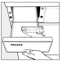
Pull the container out of the machine, gripping it firmly with both hands.
